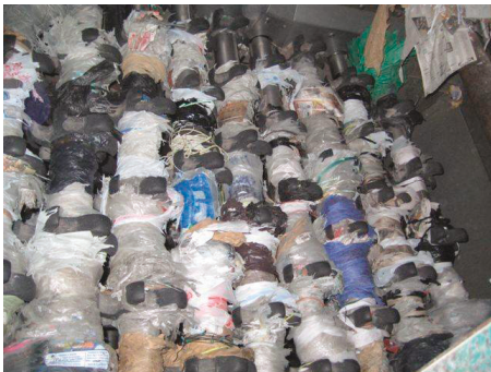
Plastic bags clog the sorting equipment at a Portland recycling facility.
